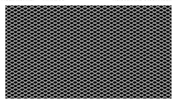
LW Pitch:6.00mmStrand Width:1.20mmSW Pitch:4.25mmThickness:1.00mmWeight:4.42 kg / m2Open Area:43%
